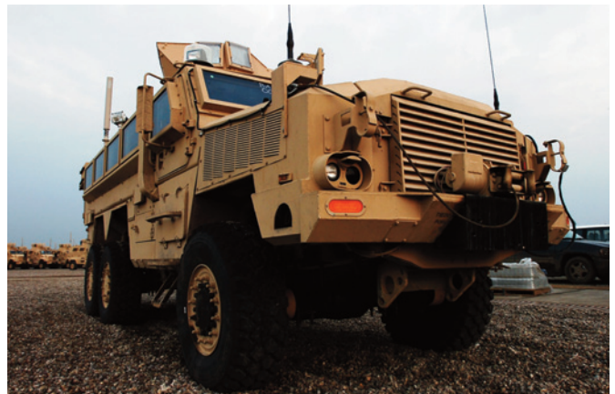
The Mine Resistant Ambush Protected Heavy Armored Ground Ambulance is the newest vehicle in a new fleet of MRAP being fielded into Iraq. (U.S. Army photo by Spc. Angel D. Martinez, 113th Mobile Public Affairs Detachment)
